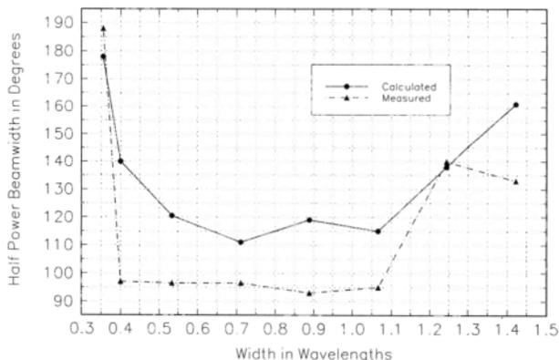
FIG. 5. Azimuthal beamwidth versus baffle width in wavelengths.
