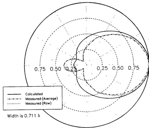
FIG. 2. Polar diagram of the amplitude response in the azimuthal plane. Baffle dimensions: 61 cm wide  $\times$  30.5 cm high. Frequency: 400 Hz. Radial scale is linear in amplitude.
