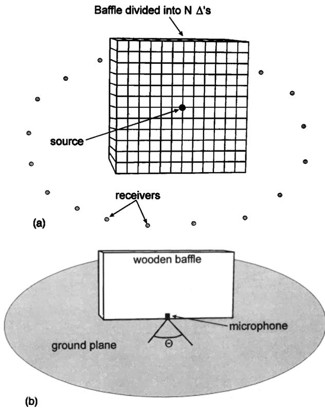
FIG. 1. (a) The configuration assumed for the computations, showing the grid for the method of moments. The receivers are assumed to be in the far field. (b) The configuration used in the physical experiments.
