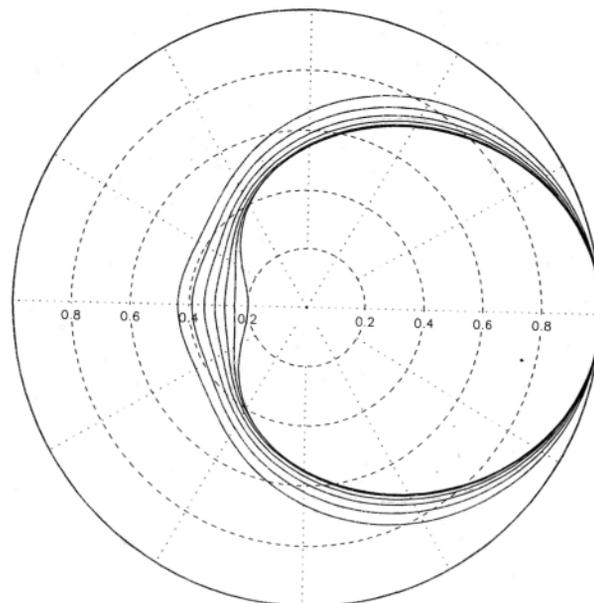
FIG. 6. Effect on amplitude beam pattern of microphone distance from the baffle. Inner curve: zero spacing. Outer curve: 15.2 cm. Interval: 2.5 cm.
